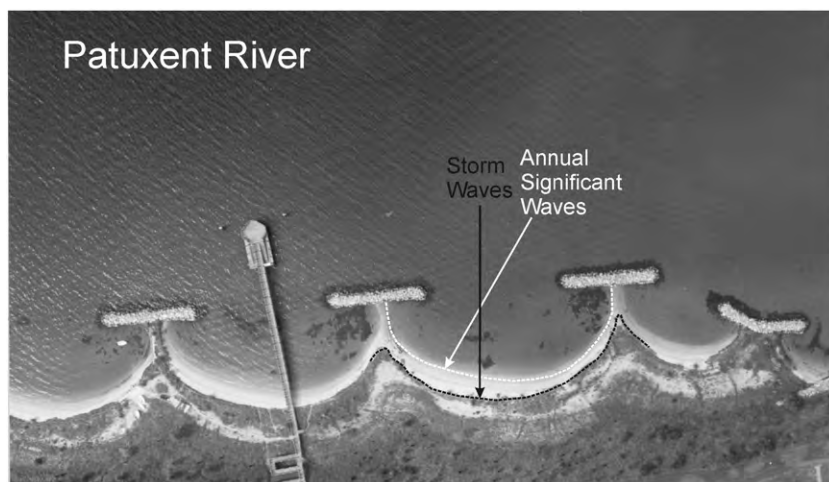
Fig. 9. Asbury project located in a coastal embayment with a unidirectional wind/wave climate demonstrating shore planforms resulting from annual and storm waves which approach from the same quadrant. Photo date: 20 Oct 2005.
