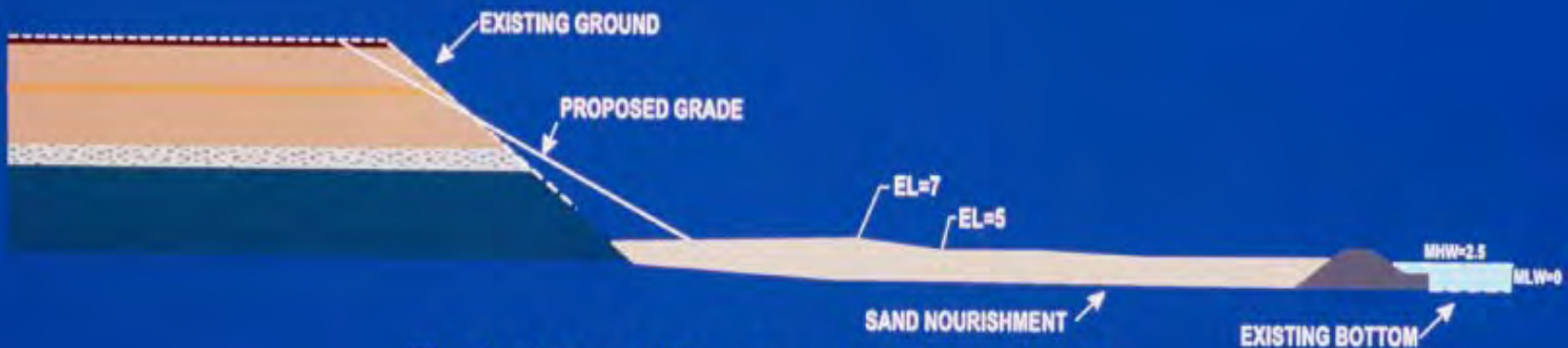
Typical Beach/Breakwater Cross Section
